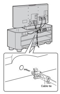
**3** Bundle the cables, and then insert the end of the cable tie through the slit of the cable tie.
